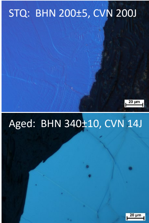
Figure 1. Microstructure at Charpy fracture surface in the (upper) solution treated condition and (lower) aged condition
